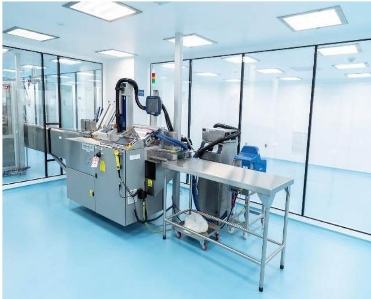
Tube filling equipment for semi-solid production line
