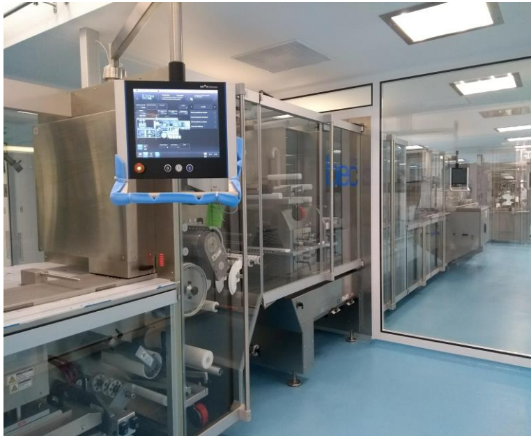
Equipment installed at OTC Plant Uhlmann Bec 700 Blister Machine Solids Production Line
